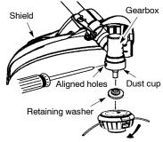
**NOTE:** Make sure all parts are properly installed as shown in the illustration before installing the trimmer head.
